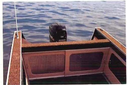
Sliding doors to gas tank and storage area
