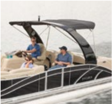
SPORT ARCH This acrylic shade features a retractable Bimini top to provide protection from the sun. Optional on Mandalay Sportlounger models and S-Series models.
