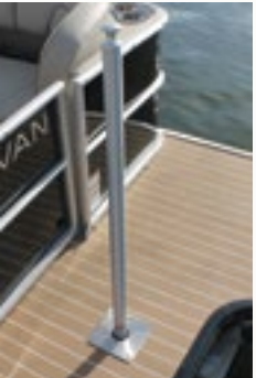
SKI PYLON Jump into water sports with a removable ski pylon that's bolted through the deck for maximum strength.
