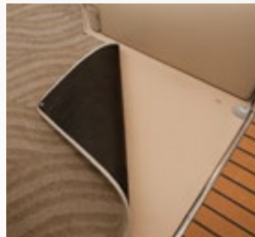
VINYL FLOOR WITH SNAP-IN CARPET The vinyl flooring stands up to wear and cleans easily after fishing. Simply snap the carpet back in place for cruising.
