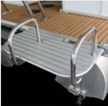
EXTENDED SWIM PLATFORM Through-bolted and braced to the deck, this sturdy extended swim platform is perfect for water sports.
