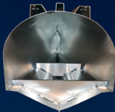
RPT 2.0 | Made of .100 gauge aluminum and a reinforced nose that incorporates a double bulkhead, rib channel system, and a strut on the seam. This third generation RPT tube design is built for high horsepower engines and is backed by a Lifetime Warranty.
