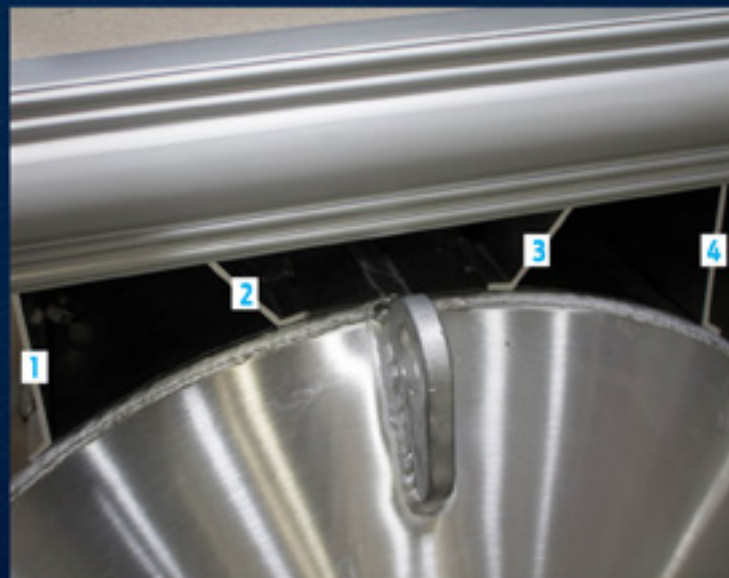
4-PT Deck to Hull Fusion | Sylvan deck brackets have 4 points of fusion for an extended area of contact with the tube. In addition to providing increased strength and support, this reduces frame twist and racking in rough water and guards against tube fatigue.
