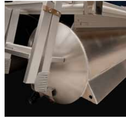
Performance Strakes | Get faster planing, better cornering and a smoother ride (not available with RPT Tubes).
